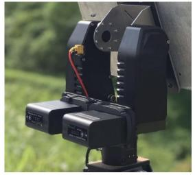
2. The antenna has to be mounted on the our AAT with the use of a special bracket. In order to prevent tampering with the normal operation of the compass built into the our AAT it is recommended to avoid using antennas made with ferromagnetic materials. Wherever possible, use non-magnetic stainless steel bolts, aluminum and other non-magnetic materials.
