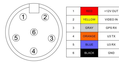
If you wish to use MAVLink protocol to provide tracking data through digital radio link: Fix the digital radio link on the antenna bracket. Connect the black wire of the plug cable to the ground wire of the digital radio link. Connect the red wire to the power wire of the digital radio link.
